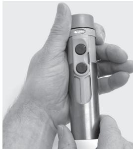
2. Grasp the device by the top and pull off the titanium sleeve.
