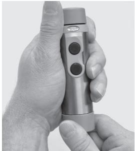
1. Unscrew the bottom cover and remove the battery holder.
